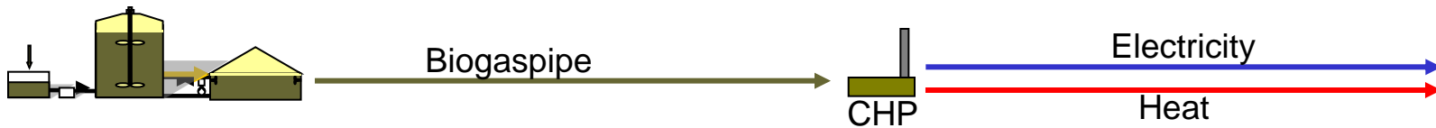
Transport of biogas
